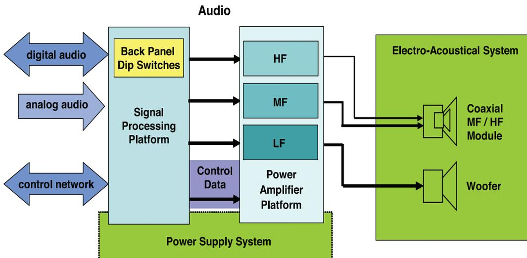
**Figure 3: Main building blocks of Genelec 8260A loudspeaker.**
