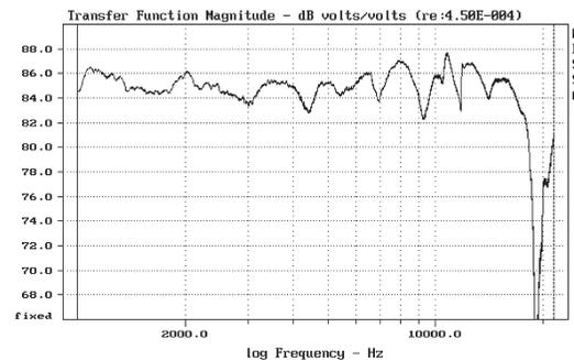
**Figure 1: Frequency response of a typical coaxial driver. Frequency response from 1kHz to 20kHz.**
