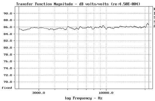
**Figure 2: On-axis frequency response of the Genelec MDC driver. Frequency response from 2kHz to 20kHz.**
