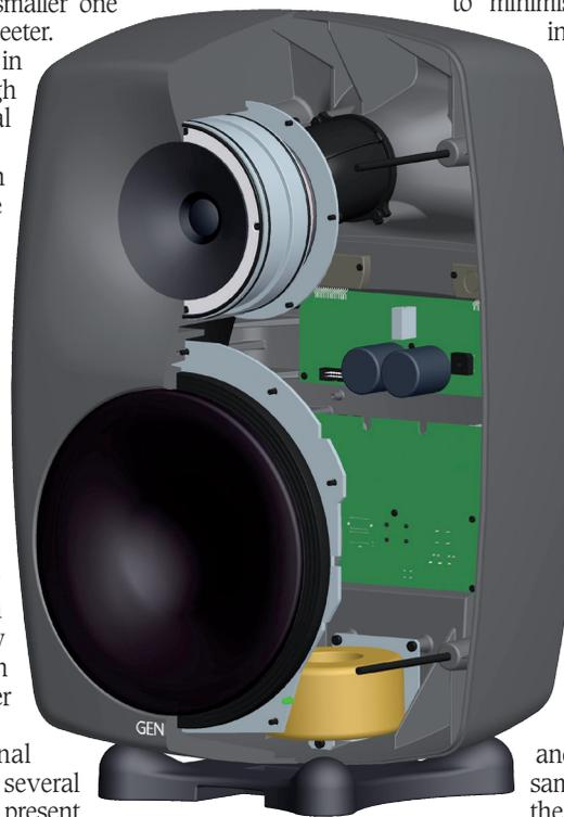
THE GENELEC MDC — The first step was to minimise the cone displacement; in other words to limit the low frequency bandwidth of the driver. This is both trivial and simultaneously important for the accepted solutions. Avoiding the sources of diffraction was more complicated. The solution resulted in several ideas, some of which are now included in the MDC driver.
